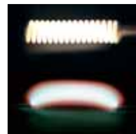
The filament of a halogen lamp compared to the arc of a XENARC® lamp.
