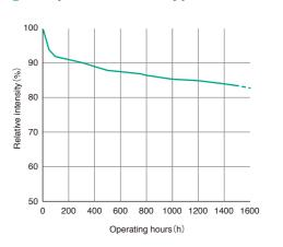
※9 Horizontal luminous intensity at continuous use. Frequent switch may cause shorter life.
